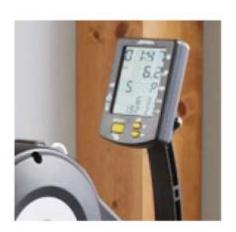
CONSOLE DISPLAYS: Measures Output, Level, Calories Burned, Calories/Hour, Time, Speed, Pulse, RPM
